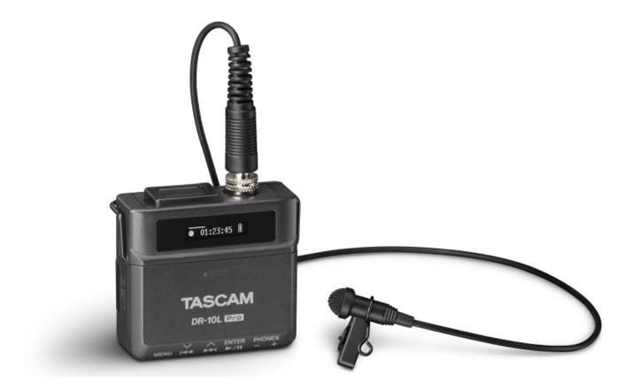
TASCAM announces the V2.0 firmware update for the company's DR-10L Pro Ultra-Compact 32-bit Float Audio Field Recorder with Lavalier Mic. Key to this update is the ability of the DR-10L Pro to accept LTC (Linear Timecode) Jam Sync and take advantage of the capabilities provided by such action. Jam Sync is the industry term for "jamming" timecode into a device so that one can link their recorder with various timecode generators.
