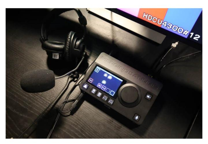
When operating the unit, both commentators can control their access to the On-Air output, can Mute their microphone (Cough Cut) and can talk to up to 4 available Talkback outputs. All these controls can be configured to be hidden, locked, latch/press-release, renamed, to offer an as safe and easy to operate experience. Various monitoring options are also available to customize the monitoring behavior when operating these controls.
