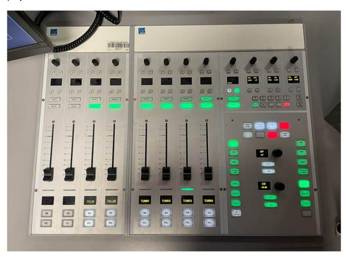
In addition to the ruby mixing consoles, MAP's radio studios are fitted with Lawo Power Core DSP mixing engines and I/O nodes. These integrate the studios with adjacent voice booths, called "studettes"; the setup then interlinks the studios and studettes with MAP's large Grand Studio with just the push of a button.
