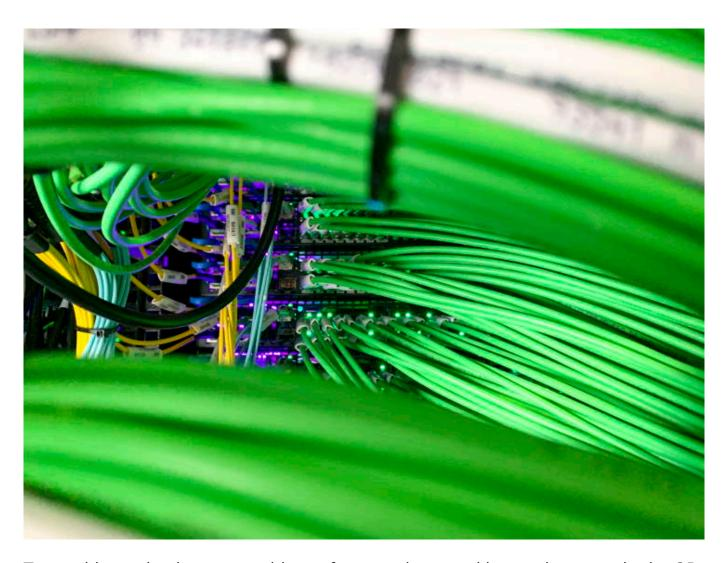
To provide production crews with a safe, spread-out working environment in the OB van's control room, Studio Berlin housed ten racks of complete equipment in a separate trailer, with a fiber optic interlink connecting the two. To save additional space, Riedel's flexible MediorNet MicroN UHD system is split between the two vehicles. As a result, the Ü10 can accommodate up to 26 workstations - and 24 UHD cameras - while maintaining a maximum distance between them.
