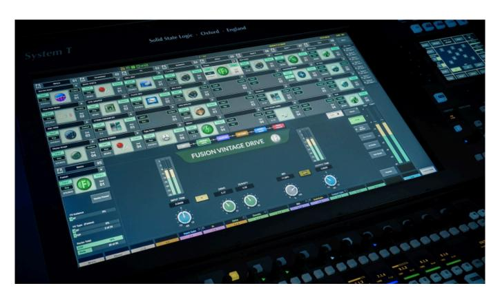
The Tempest Control App (TCA) delivers the full System T feature set and interface, offering flexible installation options provided by the separation of the control elements. With V4.1, a new dual-screen Channel View allows simultaneous control of 32 paths, while adding two Desktop Fader Tiles enables powerful, compact configurations to be built into portable, remote or desktop installations.
