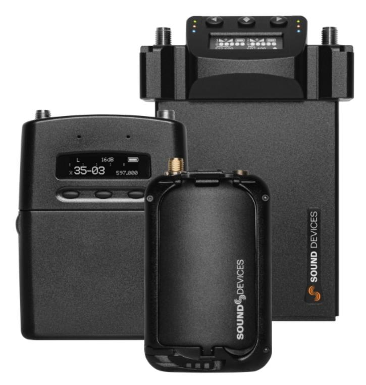
Sound Devices is shipping the A20-RX: a two channel, true diversity receiver with industry-exclusive SpectraBand technology. SpectraBand gives the A20-RX receiver and A20-Mini transmitter an unprecedented tuning range: 470 MHz - 1525 MHz. The A20-RX also features high-discrimination front end filtering for better performance in noisy RF environments and Frequency AutoAssign for faster setup. The receiver is compatible with both A20-Mini and A10-TX transmitters. Sound professionals with
