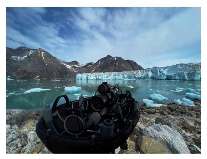
Beverly used some additional MKH 8020 mics supplied by Sennheiser specially for the Greenland expedition in spaced omni set-ups in various configurations, recording the calving of glaciers, icebergs breaking up and other unique sounds. "Apart from my Sennheiser double mid-side rig, I now also have four MKH 8020s, which I can use in spaced omni set-ups, so I'll either use them in stereo pairs or in Ouad.
