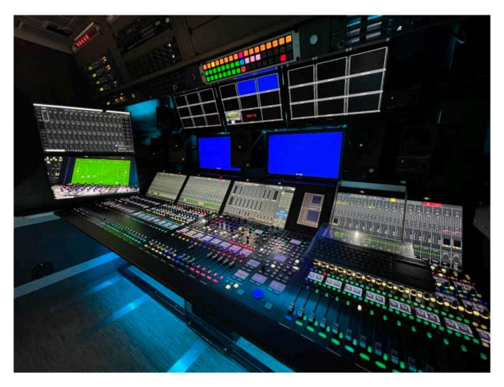
Audio Control Room 2 is equipped with a 16-fader Lawo mc<sup>2</sup>36. Its built-in A\_\_UHD core technology provides 256 processing channels (48/96kHz), local I/O, 864 channels and integrates with solutions such as Waves SuperRack SoundGrid. It also and supports ST2110, AES67, RAVENNA and Ember+. The mc<sup>2</sup>36 also offers intuitive IP network management based on Lawo's HOME platform.
