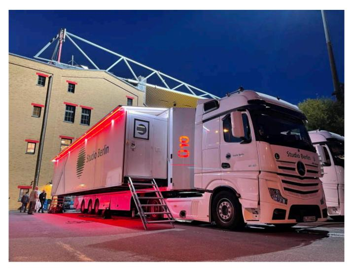
German TV production service provider Studio Berlin has commissioned a new UHD/HDR OB truck called "Ü10", outfitted with Lawo mixing consoles and control systems. Audio Control Rooms 1 and 2 of the new OB van are equipped with an mc²56 production console and an mc²36 all-in-one console, respectively, powered by fully redundant A\_UHD mixing cores and a Lawo VSM broadcast control system. Planning and construction of the vehicle was accomplished by German system integrator Broadcast Solutions.
