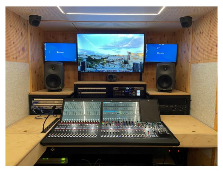
Demands on the monitoring environment are high, so a superstructure with very elaborate acoustical treatment was mounted on a truck chassis, with the outer shell and interior isolated from each other and fitted with thick, 10cm insulation. Designed for "immersive audio", the truck can accommodate mixing for Dolby Atmos and is fitted with a 7.1.4 sound system.
