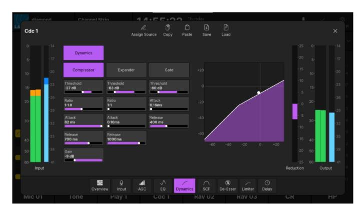
For the Power Core DSP engine, refinements include extended "Q" values to help fine-tune EQ curves, a self-keyed side-chain filter for dynamics processing which excludes frequencies from its calculations, the ability to adjust the DeEsser's active frequency, and support for up to 8 AutoMix groups – a boon for morning show and talkshow producers.
