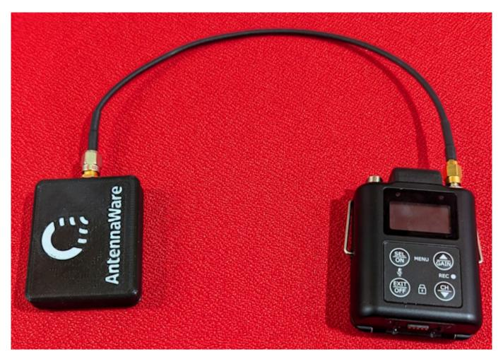
Launched at IBC 2024, the Sub-GHz BodyWave antenna promises notable increases in wireless range and reliability of signal in a form factor designed specifically to be compatible with virtually all bodyworn UHF transmitter packs.
