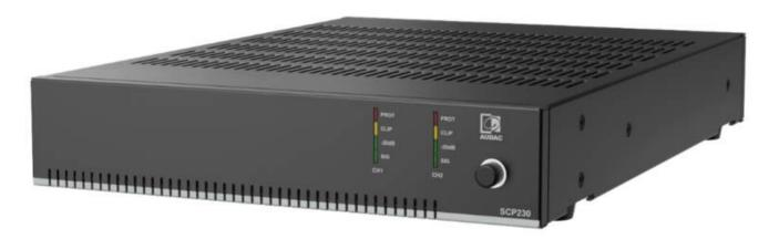
Belgian pro audio manufacturer AUDAC is announcing a new range of extremely powerful compact dual-channel power amplifiers for commercial use. These half 19" devices can be used in stereo low impedance or 70V / 100V bridge mode. There are 3 different models to serve a wide range of applications with power ratings that vary between 240W up to 600W in a half 19" rack space housing.
