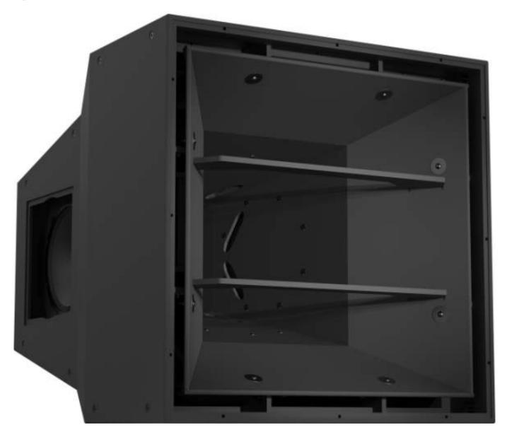
Electro-Voice is expanding its portfolio of sound solutions for stadiums and sports venues with the global introduction of the MTS series of full-range, high-output, long-throw, point-source loudspeaker systems. Each MTS model is equipped with four 15" woofers and dual coaxial mid/high frequency compression drivers. The system is capable of generating more than 151 dB peak SPL with exact directivity for very-long-throw applications.
