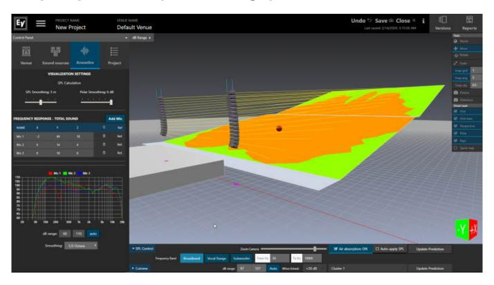
Electro-Voice is pleased to introduce PREVIEW, a new platform-independent software application designed to configure Electro-Voice line-array loudspeakers for optimized coverage. The software provides efficient system setup by creating visualizations of coverage, SPL, frequency response and precise mechanical load calculations.
