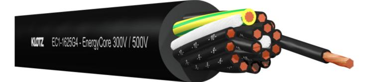
The EC1-1625G4 Energy Multicore has been specially developed for mobile event, production and media applications indoors and outdoors in accordance with DIN 15765. It is equipped with 16 x 2.5 mm<sup>2</sup> current cores and a 4.0 mm<sup>2</sup> PE protective earth in accordance with IEC 60228 (class 6) with a short strand lay length.
