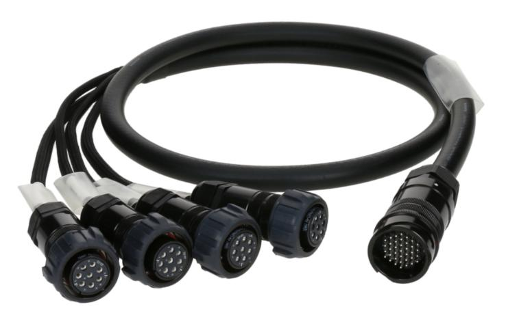
The KLOTZ LSC3215YS, specifically designed for multi-channel systems, is likely the highest quality and most durable 32-way speaker multicore on the market, purposely built for demanding live environments. Featuring 32 numbered cores of bare stranded copper wire (class 6, VDE 0295) each with a cross-section of 1.5 mm², and an exceptionally tough PVC outer jacket with liquid crystal polymer (Vectran™) braiding, it serves as the ideal basis for our premium LP321XY speaker multicore series.
