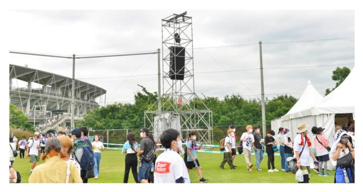
Generally, delay towers are set symmetrically to provide coverage for both sides. However, these were positioned only for coverage on one wing in order to reduce the spill to the neighbouring residential area. The result was amazing. There was no difference in sound level, starting at the FOH mix position and sufficient power was distributed across the entire venue, meeting the required SPL and quality of sound.
