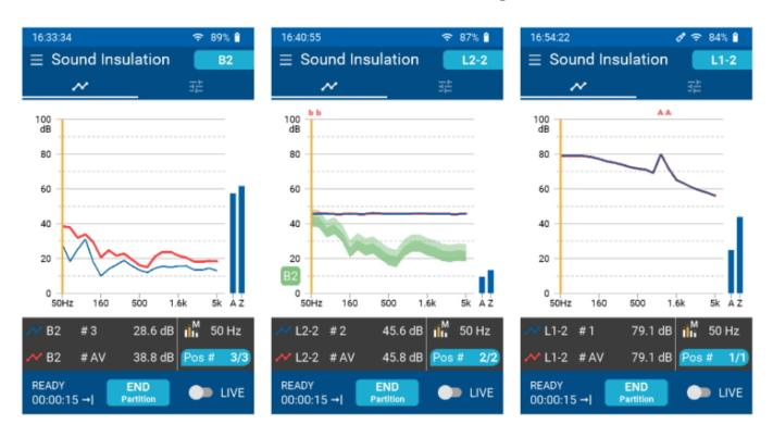
Firmware V1.42 of the XL3 Acoustic Analyzer brings a comprehensively revised user interface that significantly simplifies sound insulation measurements. All third-octave levels in the transmitting and receiving rooms are now displayed as line graphics. This enables intuitive visual recording of the spectrum and also allows multiple levels and reference values to be displayed simultaneously - for even faster and more efficient analyses.
