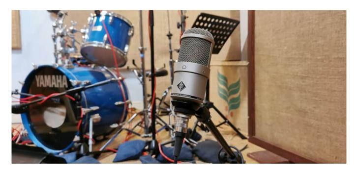
A Neumann M 147 Tube condenser microphone is used as a general mic to capture the body of an instrument, which Onabulé also uses on the double bass. For piano, a matched pair of Neumann TLM 170 large-diaphragm condenser microphones are used, which he has also found perfect for traditional classical recording.
