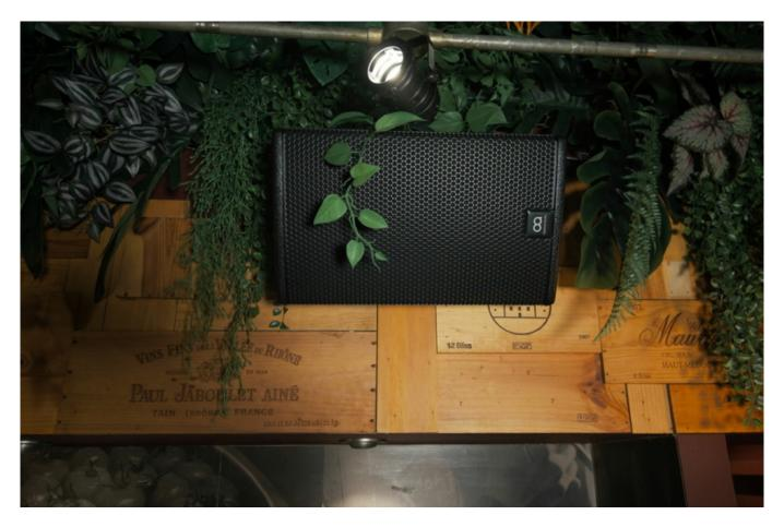
Cuboid 8 features an 8" low frequency driver for impressive punch and midband with a 1? exit high frequency compression driver for clarity of vocal and high frequency projection. The HF section delivers consistent coverage in either plane from a user-rotatable horn. Mark Blackwell, Definition Audio Visual commented: "Rich and detailed sound quality at a very competitive price point makes the Cuboid series a highly attractive option for venues like LIVIN'Italy."
