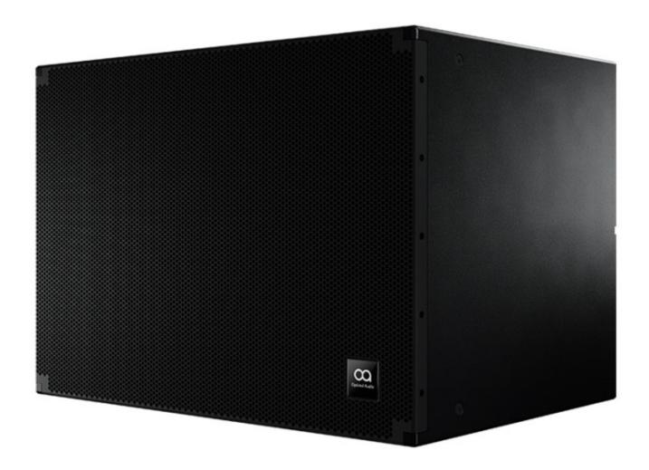
Sub 18 is a powerful, high-performance, passive, 18" subwoofer designed for applications that call for increased impact and low frequency performance across the Optimal Audio loudspeaker range. The 18" (460mm) driver is loaded into a plywood bass-reflex cabinet that maximises performance, with a peak SPL of 136dB, while taking up minimal space. Sub 18 can be used on the ground or flown using integral M8 inserts.
