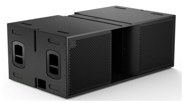
PK Sound, the robotic line array company, has formally released the T218 intelligent subwoofer. Onboard DSP, class-D amplification, and networking enable auto-identification and configuration within PK .dynamics software through a simple multipin connection. Dual front-loaded, 18" long-excursion transducers in a bass reflex design achieve a peak output of 144dB with an operating range of 25-100 Hz for clean and impactful low-frequency performance.
