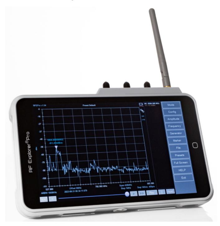
RF Venue has extended its portfolio of wireless audio essentials with the addition of the RF Explorer Pro, a touchscreen RF spectrum analyzer configured for wireless microphone and in-ear monitor system users. With its integrated 6 GHz Spectrum Analyzer and Frequency Coordination and WiFi Analysis tools, RF Explorer Pro offers advanced functionality with intuitive touchscreen operation to maximize the performance of wireless microphone and in-ear monitor systems in any venue.
