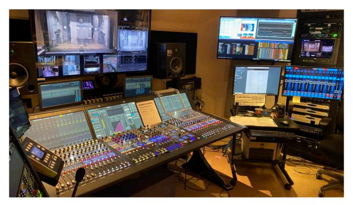
"One big challenge with the previous equipment was lack of DSP, which required a lot of outboard processing gear," Mitchell explains. "Since we had previously installed AoIP infrastructure with our first Lawo console, it was easy to replace the old stageboxes with the Lawo A stage64 using existing wiring, and adding the
