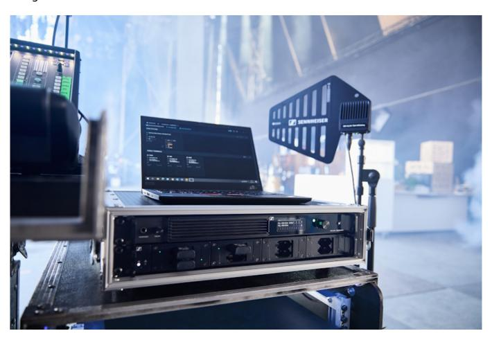
Spectera's wideband approach allows IEMs and mics to share the same TV channel, automatically coordinating all packs. The system constantly senses and adapts, so engineers don't need to wrestle with calculations or worry about local interference. "The noise floor was around -80 dBm. One cool feature is that it measures the noise floor while transmitting, so you can see what you're working over," Vaughn notes.
