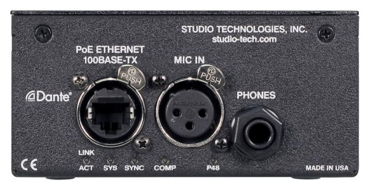
Set up and operation of the Model 203 is simple. An etherCON RJ45 jack is used to interconnect with a standard twisted-pair Ethernet port associated with a PoE-enabled network switch. This connection provides both power and bidirectional digital audio. A broadcast headset or handheld ("stick") microphone can be directly connected to the unit's 3-pin XLR microphone input connector. A ¼-inch 3-conductor (stereo) jack is used to connect to selected headset, headphones, or an earpiece.
