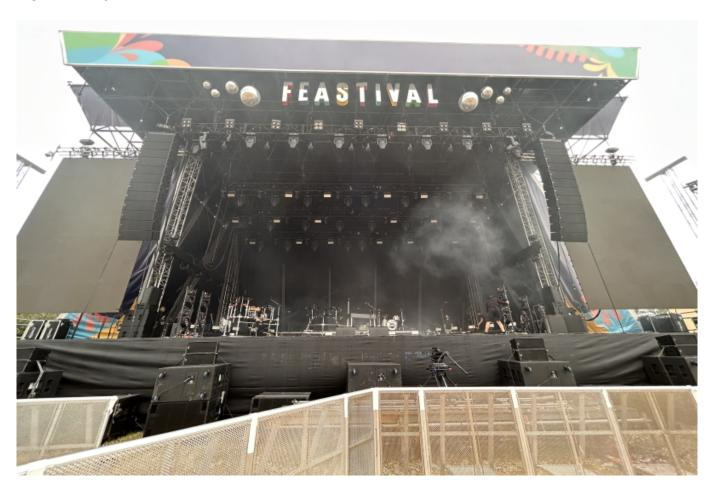
WPL was driven in 2-box resolution from Martin Audio's process-controlled multichannel iKON amps, and by using Martin Audio's new DX4.0 dedicated system controller, they were able to place the legacy W8LC on the same network, allowing full system control from a single point. A further eight W8LM along the stage lip provided front fills and  $12 \times XE500$  wedges were available to provide additional stage energy. Also providing premium stage fills on each side were a pair of TORUS
