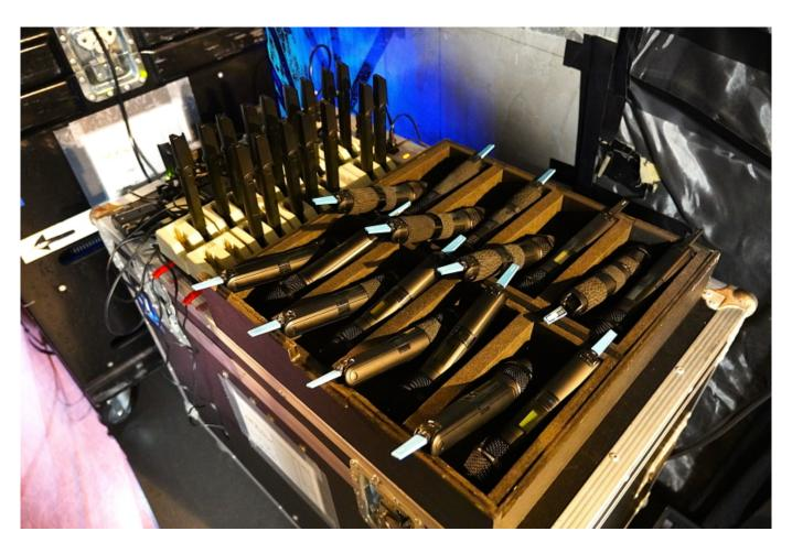
One of the reasons the 6000 Series was used for One Step is its stable connectivity as demonstrated in areas with RF interference, as Masaru explains: "We expected that the Expo venue would have an incredible amount of RF from different stages within a small area. I wanted to use the 6000 Series from the start because we know it's the most stable wireless system and we have trust in this product based on our past experiences."
