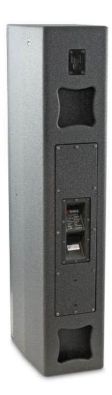
Like the other TENNAX family members, the Powerstick-6 is made of high-quality birch multiplex, CNC milled, grooved, waterproof glued, screwed and coated with weather resistant Polyurea. It also offers various M10 thread points, swivel brackets, wall and mast brackets as well as a Safety Point for a Single Stud for easy setup.
