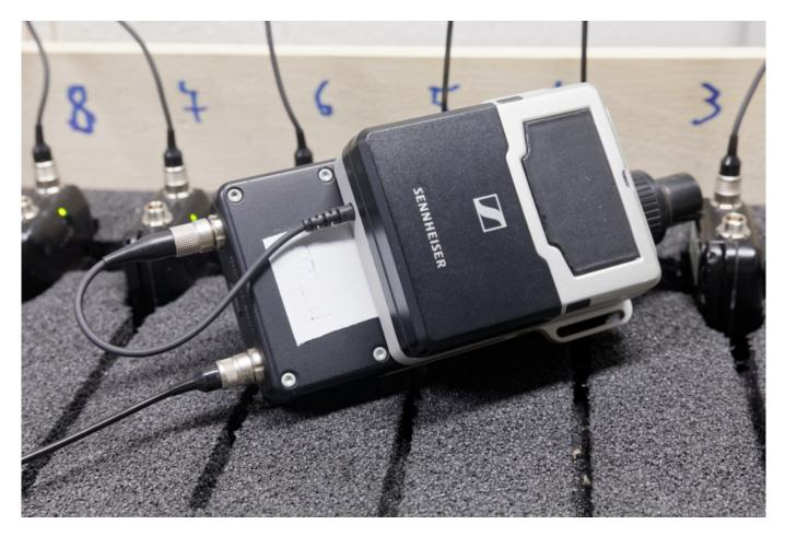
The 32 digital channels available at the Munich Kammerspiele are used with ultracompact SK 6212 bodypack transmitters. Four SK 6000 are also available, and are used in combination with an adapter to enable conventionalmicrophones to be operated wirelessly in a similar way to using an SKP plug-on transmitter. This special solution ("P48 Phantom Power Adapter for SK 6000/9000") with an XLR connector and lock ring provides 48 V phantom power and in the meantime is also
