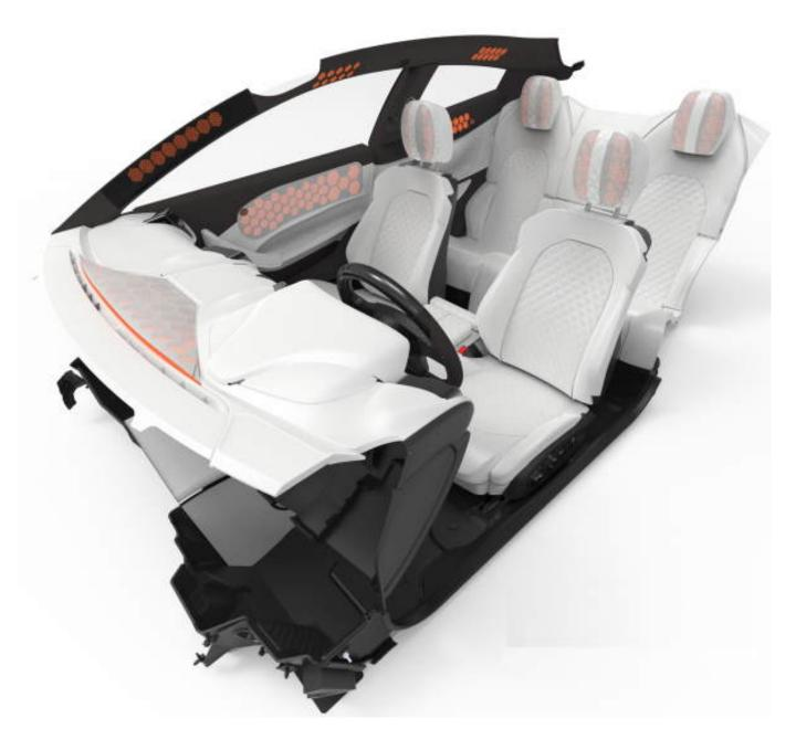
Warwick Acoustics' ElectroAcoustic Panels bring significant whole vehicle system benefits compared to the use of conventional audio technology. Like-for-like, ElectroAcoustic Panels are up to 75% lighter, consume up to 75% less power and offer significant interior design and packaging freedom.
