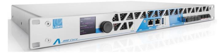
Powering both members of the mc² family is the software-defined A\_\_UHD Core Audio Engine with intuitive HOME functionality. Up to 1,024 mc²-quality DSP channels can be shared between multiple consoles based on a flexible licensing system.
