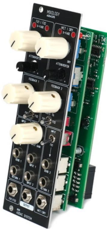
ADDAC System announces the new ADDAC815 Mixology Eurorack module, following the introduction of its Mixology pedal in December. Mixology brings powerful routing and unconventional mixing capabilities into the world of Eurorack - in a modest 10HP footprint. This module serves as both a dual effect chain router and feedbacker, and can also function much like a 3x3 matrix mixer, enabling multiple routing configurations within a very compact set up.
