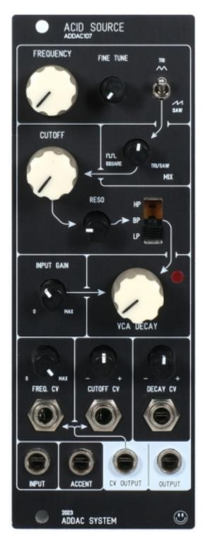
ADDAC System announces its latest Eurorack module, ADDAC107 Acid Source. Acid Source, a compact synth voice incorporating full VCO, VCF and VCA functionality, forays deep into acid sonic territory with classic 'squelchy' sounds - all of which may be shaped using its built-in low-pass, band-pass and high-pass filters. Whether being used for a plucky bass line, a squelchy lead synth line or scratchy percussion,
