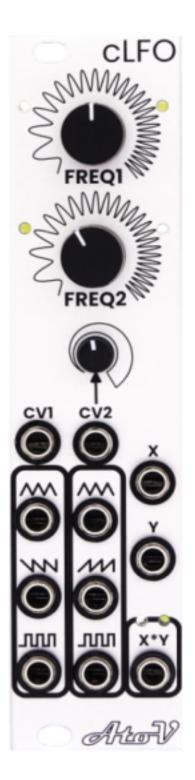
Introducing the innovative Complex Low Frequency Oscillator (cLFO). The cLFO is an instrument for those who believe in pushing the limits of modulation. Featuring two CV-controlled LFOs that intricately intermodulate and are seamlessly integrated with a ring modulator, this module elevates your synthesis and sound design to unprecedented levels. Crafted with a focus on cross and self-patching, the cLFO
