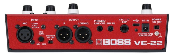
The VE-22 provides an XLR input and integrated preamp for a professional stage microphone, plus phantom power for high-end condenser types. A high/low gain switch, rear-panel sensitivity knob, and level meter enable the user to optimize the input signal for nearly any mic. USB-C, an analog aux input, and a headphone jack support a variety of vocal activities, including daily practice, computer recording, music playback from a smartphone, and livestreaming on social media.
