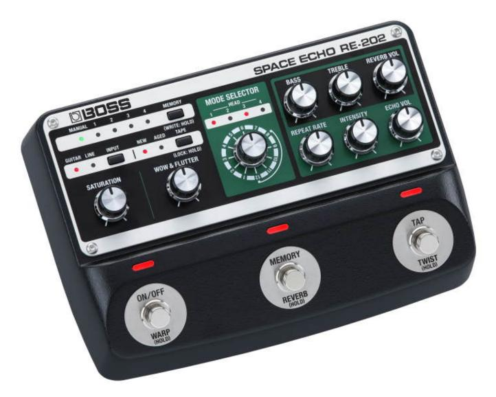
The RE-202 delivers the full vintage vibe of the RE-201 - without the need for regular tape replacement and hardware maintenance. All the core controls of the original are here, including the iconic 12-position mode selector. Every behavior is replicated with complete accuracy, such as the gradual pitch change that occurs when the Repeat Rate knob is tweaked, or the cool runaway feedback that happens when the Intensity knob is maxed.
