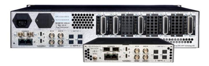
Right out of the box, Core 256 comes with a total of 592 input and output channels across Thunderbolt, Dante, MADI and ADAT, but it can also be expanded with a MADI module, adding 128 extra channels. Finally, Core 256 comes with built-in 512x64 channels of Pro|Mon summing, SPQ Speaker EQ processing and capacity for 1,500 x 1,500 channels internal routing.
