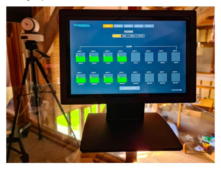
In cooperation with the British manufacturer of touch-based display solutions Densitron, DirectOut is proud to offer new control options to customers of its modular PRODIGY series. Users gain fast and intuitive access to selected parameters of the PRODIGY.MC multichannel converter and the PRODIGY.MP audio processor.
