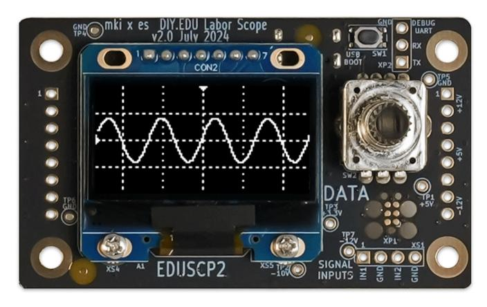
This EDU DIY Labor add-on, featuring the oscilloscope, the voltmeter, the spectrometer and the tuner, turns the, Labor into self-contained electronics development and experimentation station.
