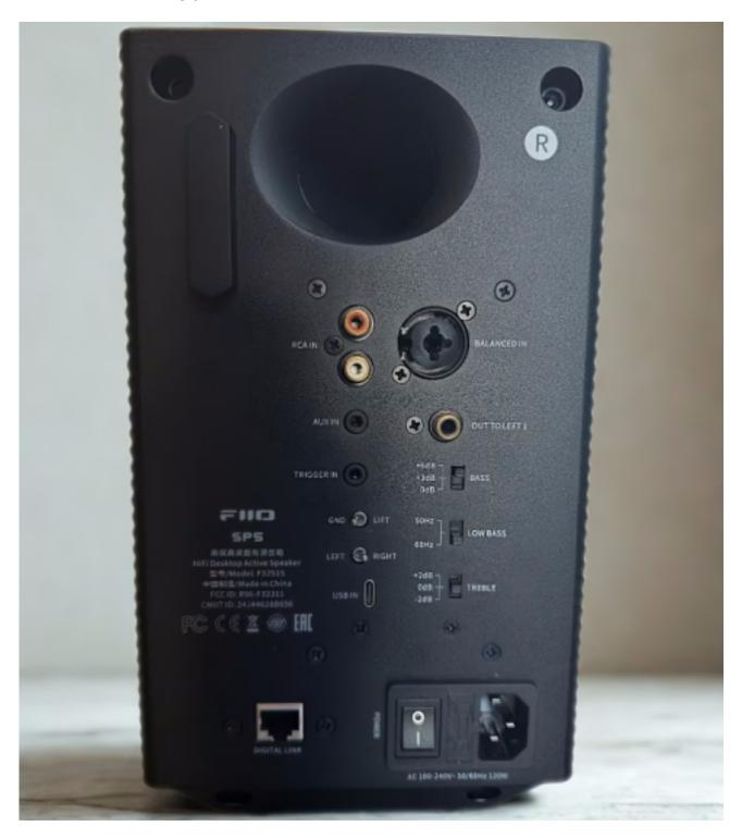
With AUX, RCA, XLR, and USB Type-C inputs, the SP5 welcomes analog and digital sources alike and all are oursupported by independent volume memory, so each input retains its own customised level settings. A low-noise, high-precision encoder enables stepless, electronic volume adjustment via the front-mounted control knob, ensuring zero loss of resolution across the spectrum. The SP5 offers full support for
