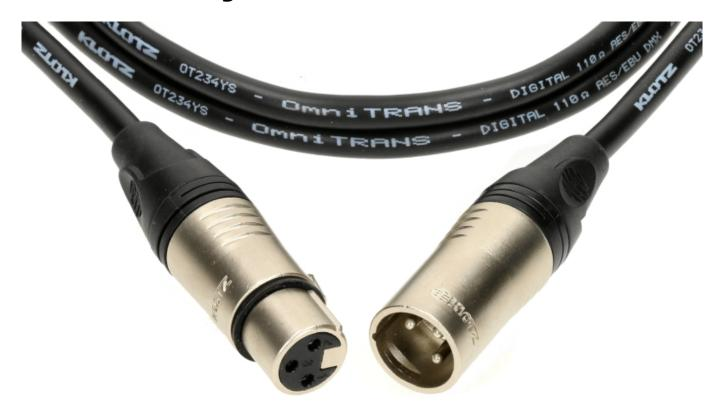
KLOTZ AIS now supplies the new PD7 Pro Digital series with the high-quality OT234YS low loss cable for AES/EBU and DMX signals. The connectors available are either the XLR 3p. and XLR 5p. plugs by KLOTZ or Neutrik. The double shielded OT234YS has a massive conductor cross-section of 0.34 mm² (AWG 22/7) and is ideal for professional applications thanks to the durable PVC jacket.
