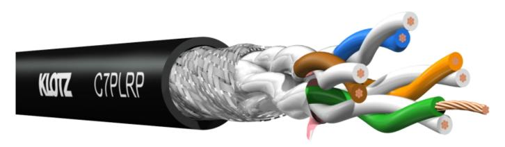
The newly developed, flexible C7PLRP network cable now enables transmission lengths of up to 100m and is therefore ideal for mobile applications that until recently were reserved for typical installation cables. Thanks to its elaborate and robust CAT7 - S/FTP - AWG23/7 - 600 MHz construction with a consistent outer braided shield and foil-shielded pairs, this KLOTZ mobile cable is the ideal choice when high reliability and fast data transmission are required.
