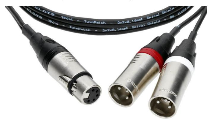
Stereo microphones are widely used in recording studios and in broadcasting. The stereo signal is provided via XLR 5p. socket on the stereo microphone. In order to connect the stereo microphones to a mixing console or a dual-mono preamp, a stereo microphone Y-cable is required, which provides the two signals (L+R) as a balanced mono microphone signal via two XLR 3p. plugs.
