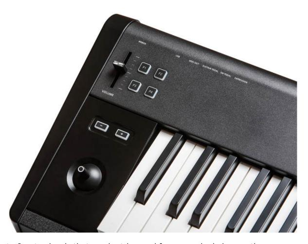
Create up to 8-note chords that can be triggered from any single key on the keyboard. Pitch and modulation can be controlled on a programmable XY Joystick. Programmable slider and six buttons permit custom controls such as volume, transposition, multi switching, zone muting and more. Assign front panel buttons to MMC Play/Stop and remotely control your DAW transport. The KM88 offers two switch pedal and one continuous controller pedal input – all user-programmable.
