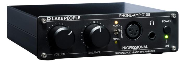
The G108 headphone amplifier from Lake People makes balanced push-pull amplifier technology available in a device designed for studio use. It enables highend headphones to perform at their peak with detailed sound and fascinating stereo localisation.
