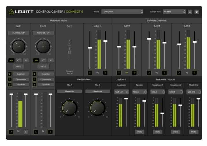
For example, Mix A could be used for personal monitoring while Mix B is being sent wherever you need it, be it your DAW, a streaming software, or a virtual meeting. You can even send your mix to applications on your mobile device. Both mix outputs feature a one-knob Maximizer to ensure that your mixes always have the optimal loudness level.
