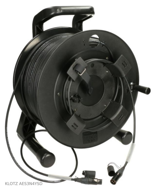
KLOTZ now supplies two new digital cable drums with high-quality Neutrik XLR 3p. and 5p. connectors with protective caps. KLOTZ uses the new OT234YS low loss data cable with a conductor cross-section of 0.34 mm<sup>2</sup> (AWG 22/7) as the digital cable.
