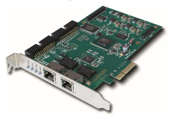
MARIAN introduces the Clara E PCle audio solution, enabling a seamless integration of audio computers in Dante networks. Digital real-time transfer of up to 1,024 uncompressed audio channels via standard Ethernet infrastructures make Dante one of the most versatile audio distribution systems. MARIAN combines this versatility with its own technology to achieve exemplary reliability.
