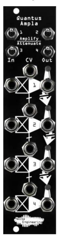
Quantus Ampla is a compact four-channel VCA. But it's not just any VCA: with some unique normalizing, mixing, and CV options, and a bit of NE flair, you can use it for tons of stuff. From the top, each channel has two independent modes: Amplify, which gives you normal VCA response, and Attenuate, which makes the VCAs close instead of open in response to positiveCV. The CV inputs are circularly normalled, so
